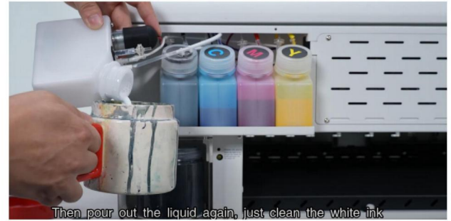
Step 20. Then pour out the liquid again, just clean the white ink bottle, because white ink has a high density and is prone to sedimentation.
