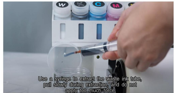
Step 20. Use a syringe to extract the waste ink tube, pull slowly during extraction, and do not apply too much force.
