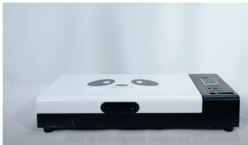
Step 5. Bake at 120 degrees Celsius for 150 seconds.
