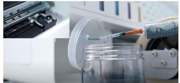
Step 12. Extract the liquid from the ink pad.
