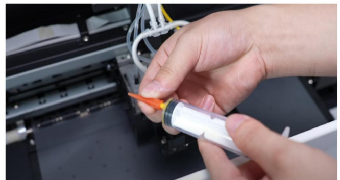
Step 16. Replace the needle with a new one when extracting different inks.
