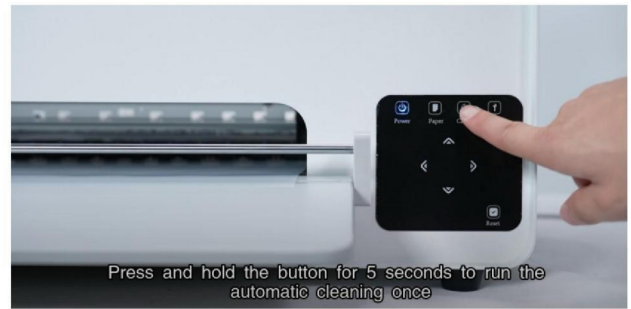
Step 26. Press and hold button for 5 seconds to run the automatic cleaning once.
