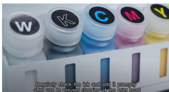
Step 9. Regularly check the ink and add it promptly after use to prevent clogging of the print head.
