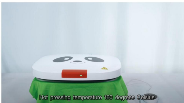
Step 3. Hot pressing temperature 160 degrees Celsius.
