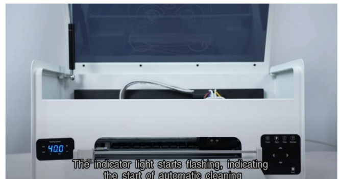
Step 24. The indicator light starts flashing, indicating the start of automatic cleaning.
