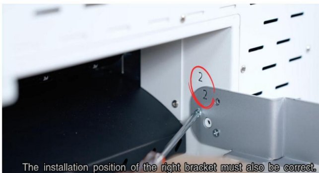
Step 23. The installation position of the right bracket must also be correct.
