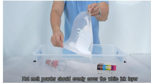
Step 2. Hot melt powder should evenly cover the white ink layer.
