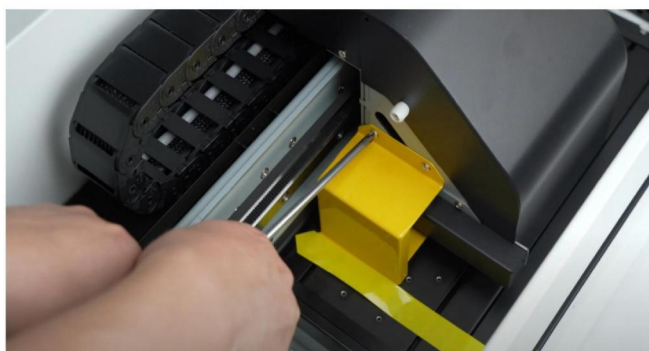
Step 13. Remove the yellow buckle that secures the ink cart.
