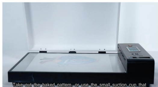
Step 9. Take out the baked pattern, or use the small suction cup that comes with the oven to remove the pattern to prevent burns.
