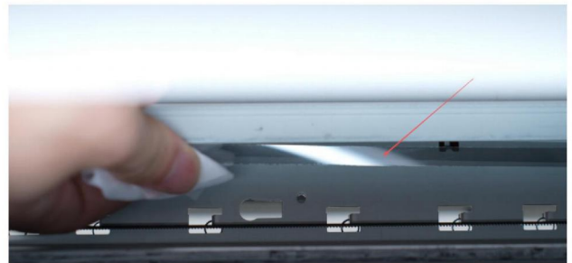
Step 22. The transparent grille strip behind the ink car can be cleaned and wiped every two weeks using a dust-free cloth.
