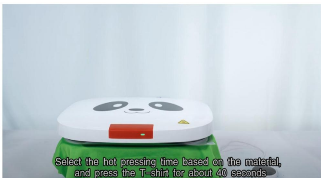
Step 7. Select the hot pressing time based on the material, and press the T-shirt for about 40 seconds.
