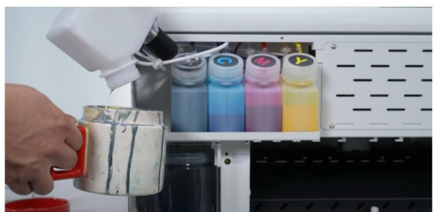
Step 16. When the white ink is almost used up, pour out the ink at the bottom.
