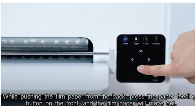
While pushing the film paper from the back, press the paper feeding button on the front, and the film paper will move out. Step 38. While pushing the film paper from the back, press the paper feeding button on the front, and the film paper will move out.
