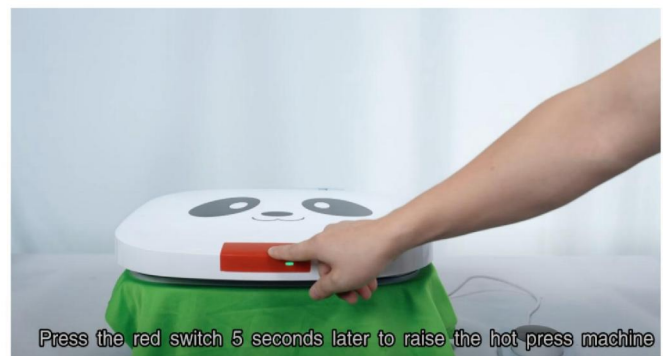
Step 4. Press the red switch 5 seconds later to raise the hot press machine.
