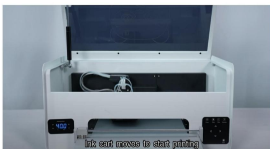
Step 7. Ink cart moves to start printing.
