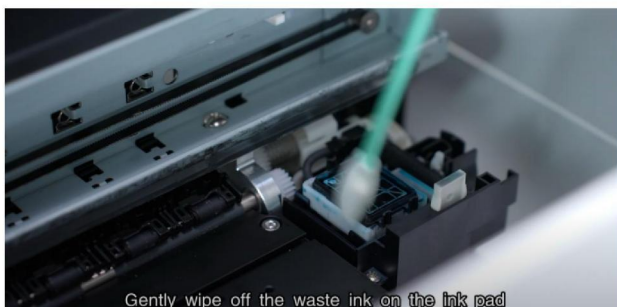
Step 7. Gently wipe off the waste ink on the ink pad.
