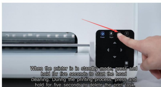
Step 7. When the printer is in standby mode, press and hold the clean button for five seconds to start the head cleaning. During the printing process, press and hold for five seconds to delete the print task.
