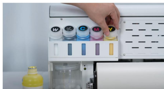
Step 8. Tighten the bottle caps after all the ink tanks are filled with ink.
