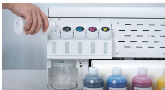
Step 7. Adding 80% to the ink bottle is enough.
