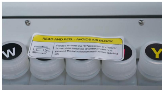
Step 3. Ensure that a no ink printing test has been conducted before adding ink
