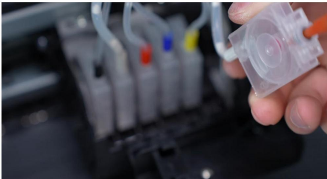
Step 13. Remove the ink sac and use a syringe to extract it.
