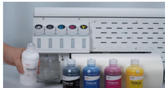
Step 4. Add the corresponding ink based on the letters on the ink bottle.
