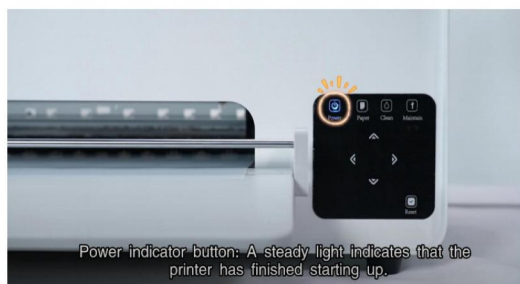
Step 5. Power indicator button: A steady light indicates that the printer has finished starting up.
