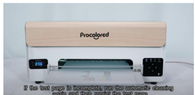
Step 32. If the test page is incomplete, run the automatic cleaning again and then reprint the test page.
