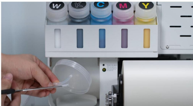
Step 19. Go to the back of the printer, take out the waste ink bottle, and cut off the zip tie.
