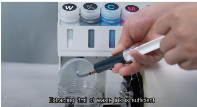
Step 21. Extracting 8ml of waste ink is sufficient.
