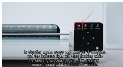
Step 8. In standby mode, press and hold for 5 seconds, and the indicator light will start flashing while the cleaning process begins. The cleaning process usually takes about 2 minutes.
