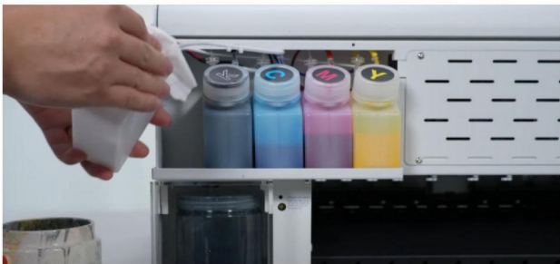
Step 21. Wipe the white ink bottle clean, then put it back, and finally add white ink again.
