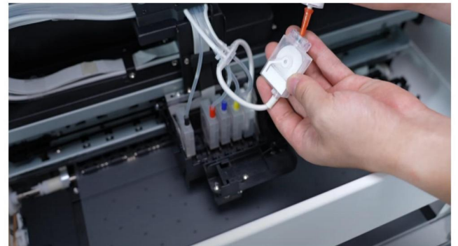
Step 14. Extract approximately 3ml of ink from each of the ink sacs.
