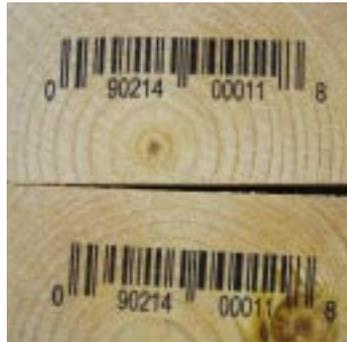
*Printing wood grade marks comprised of legible text and graphics was a situation ideally suited to the inc.jet print solution. In a lumber mill environment, a metal ski protects the inc.jet print heads and bulk ink delivery system from the harsh knocks of wood processing.*
